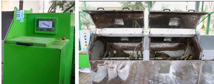
Control pannel and fermentation unit
